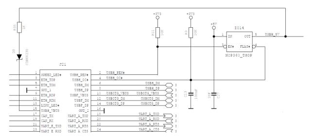
The VBUS output voltage of the USB Host interface on the Base board is connected to pin 15 of the SODIMM connector by a small schottky diode and a 1k series resistor. This circuit conforms to all CPU modules.
