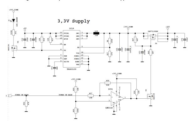
The 3.3 V supply +3V3\_DIMM is connected to the SODIMM connector. The local peripheral supply +3V3 is separated by the P-MOSFET T6 which is driven by the comparator IC21 and the N-MOSFET T5. The comparator is used since the falling slope of the signal POWER\_ON\_BASE is very slow on some CPU boards. The comparator ensures hard switching at power on and off.
