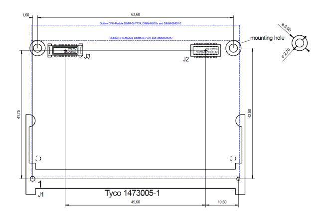
Watch: This drawing is only valid when the specified connector types are used!!
