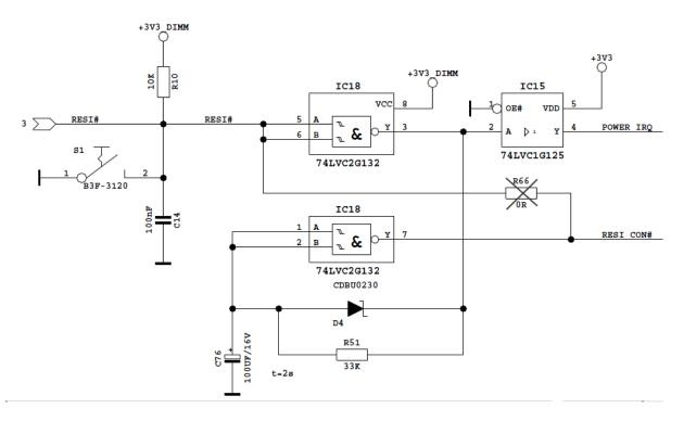
In this circuit the signal POWER\_IRQ is driven high immediately if the reset button S1 is pressed or the signal RESI# becomes low. If R66 is not fit the rising edge of POWER\_IRQ is delayed by the circuit comprised of R51, C76 and D4 and causes an active low reset signal RESI\_CON# some time later. The delay between POWER\_IRQ and RESI\_CON# becoming active can be used by the software to close the necessary tasks.
